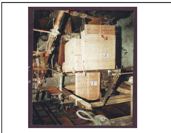
Fig. 8 : Card Binding and punched cards of plastic sheets
