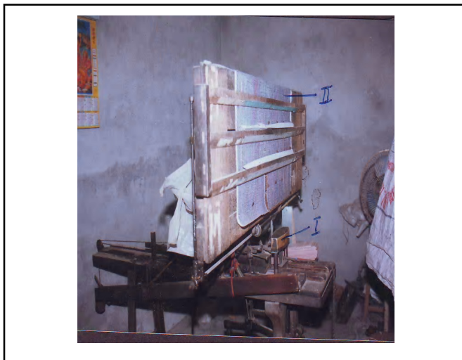
Fig. 7 : Card Punching Machine with Graph Fitted on its wooden board
