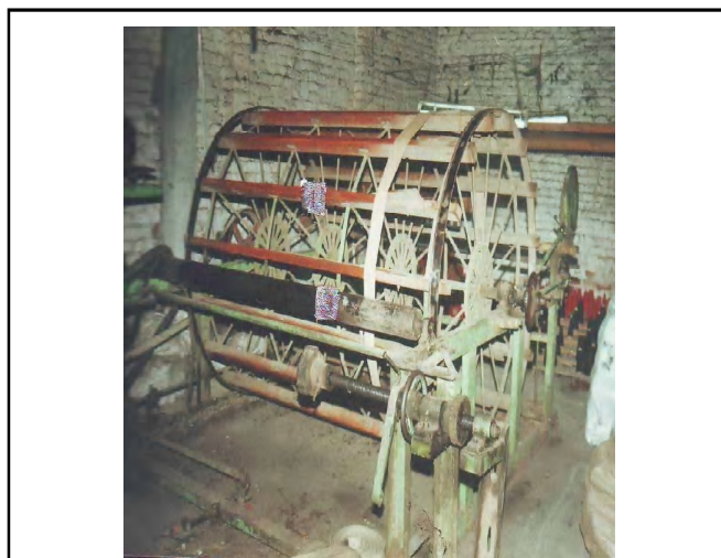
Fig. 5 : Warping Machine, its Drum and Guide Roller
